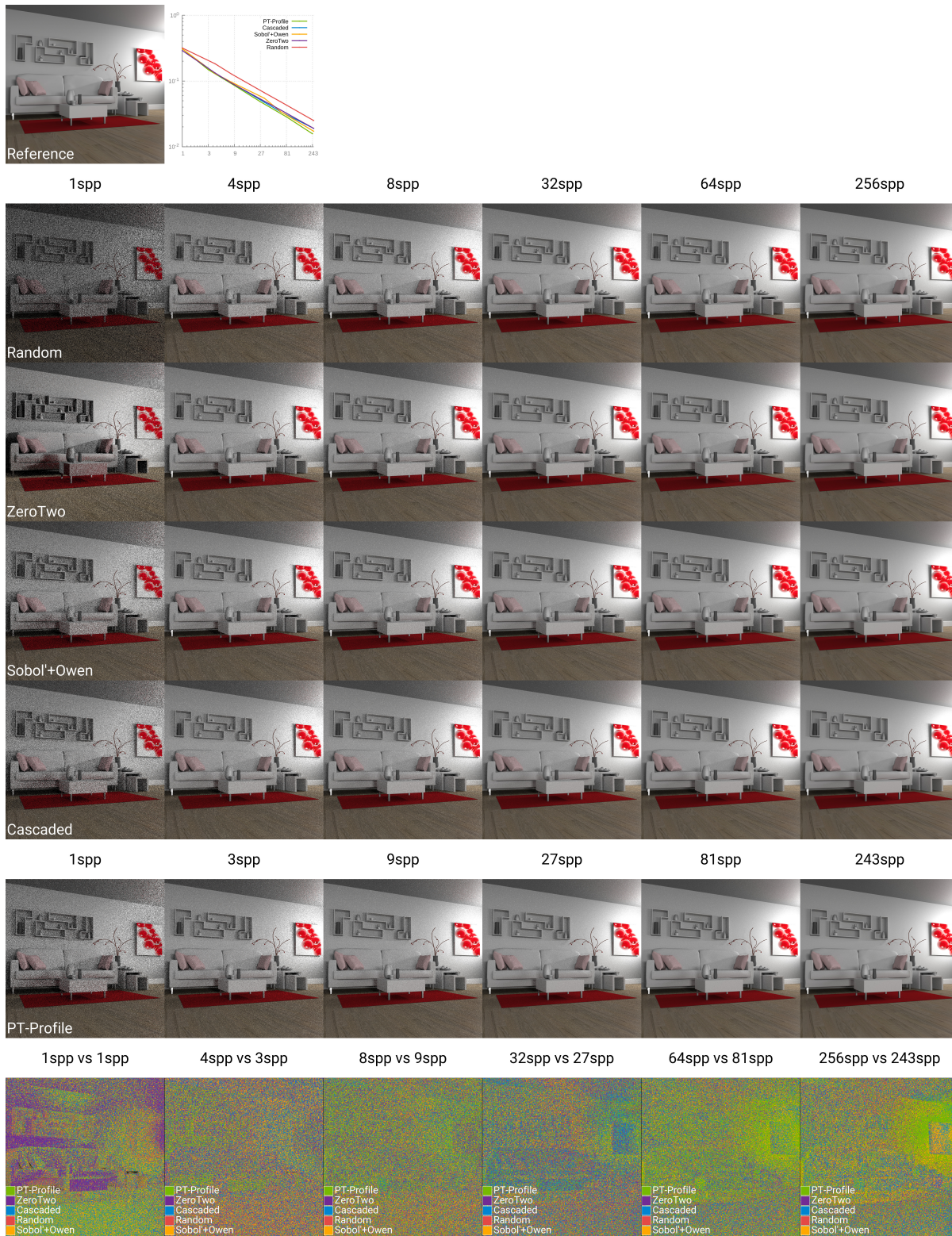
Fig. 8. Rendering results and comparisons in 8d, 3 light sources case: please refer to Fig. 7, last row in the main document. The 8 dimensions are used to sample the pixel (2d), the direct lighting (3d) and the indirect lighting (3d).
